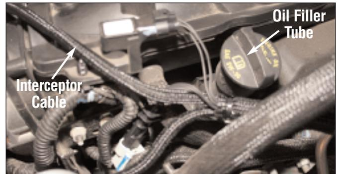
Route the Interceptor harness and all connectors away from the oil fill tube, and hold in place with provided zip-ties as necessary.
