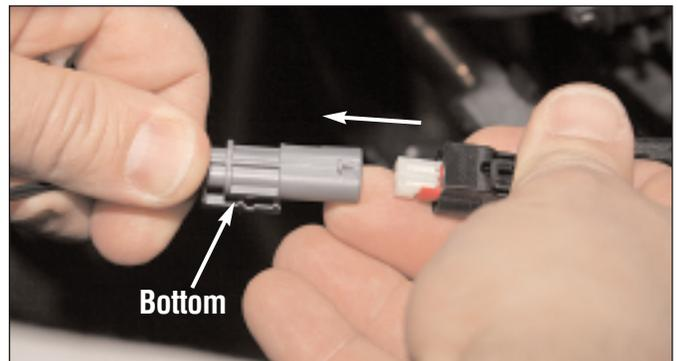
Plug the Interceptor harness 2-Pin connector into the factory wiring harness 2-Pin connector. **NOTE: The correct orientation of the connector is shown.**
