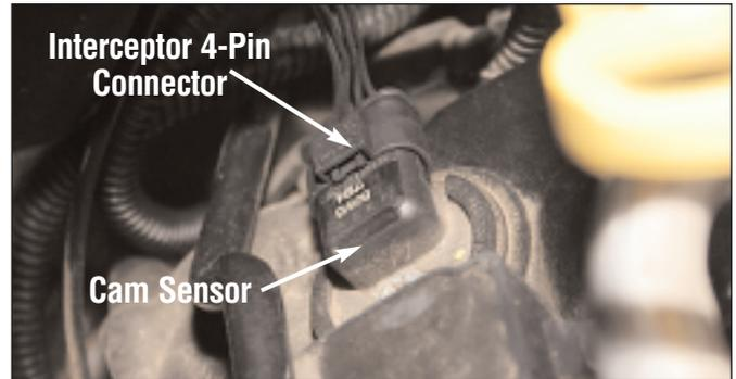
Plug the Interceptor 4-Pin connector into the vehicle cam sensor. Then plug the Interceptor harness 4-Pin connector into the factory wiring harness 4-Pin connector.
