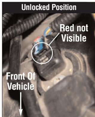
Disconnect the factory connector for the 4-Pin cam sensor. The Cam sensor is located on the passenger side behind the air intake tubing (See above photo). This connector has a locking clip that must be slid back to unlock. Notice the slight difference in the position when the tab is in the "UNLOCKED" position. Then, squeeze down the locking tab, and push the connector in slightly (toward sensor) and then remove.
