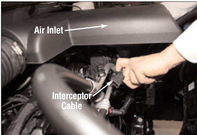
Route the Interceptor harness between the throttle body and air inlet pipe, and then back to the 4-Pin (CAM) sensor.
