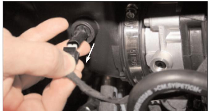
Disconnect the factory connector from the 2-Pin (Intake Air Temp) sensor. Next, plug the Interceptor 2-Pin connector into the vehicle Intake Air temp sensor.
